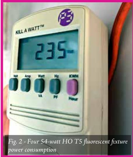
Fig. 2 - Four 54-watt HO T5 fluorescent fixture power consumption
